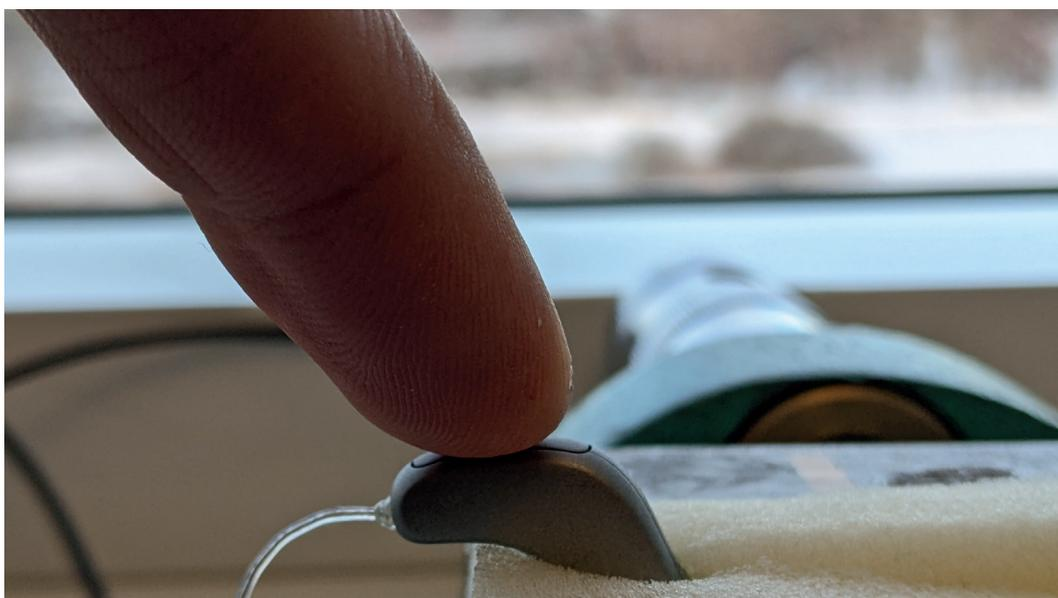
*Figure 8: The SmartRIC subjected to a finger touch in the touch noise test. The SmartRIC was connected to an acoustic coupler and routed to headphones.*
